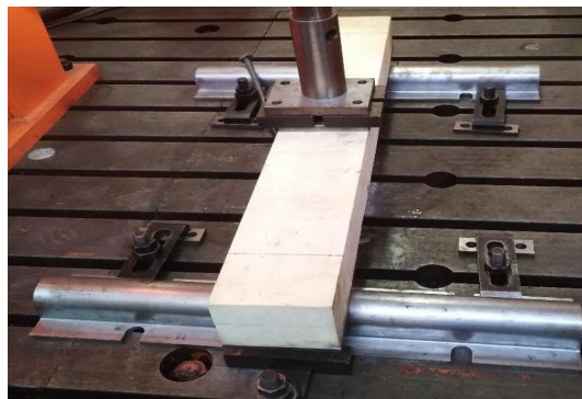
Fatigue Performance Experiment of Low Density Sleeper 低密度轨枕疲劳性能试验
