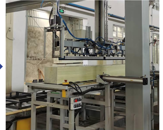
Cutting Palletizing 切割托盘
